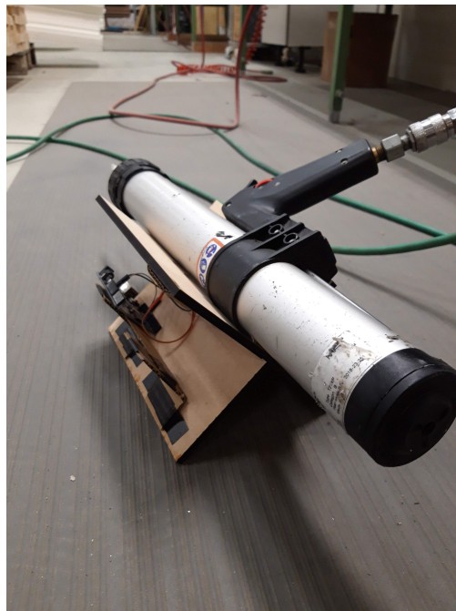
Figure 6: Laser cut docker for tool using Ultrasonic Distance Sensor.
