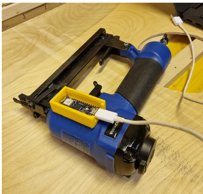
Figure 29: An Arduino on a small staple gun for the usability test.
