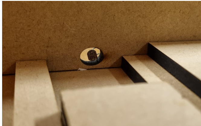
Figure 7: Photocell mounted to the mock jig for detecting lamella placement.
