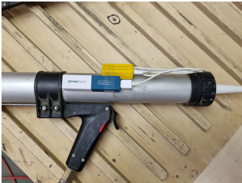
Figure 7: The pneumatic adhesive gun with the movement measuring Arduino. The Arduino slid towards the table during testing and became tilted in the y-direction, a possible error in the readings.
