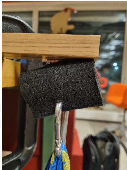
Figure 14: Setup for tensile strength test.
