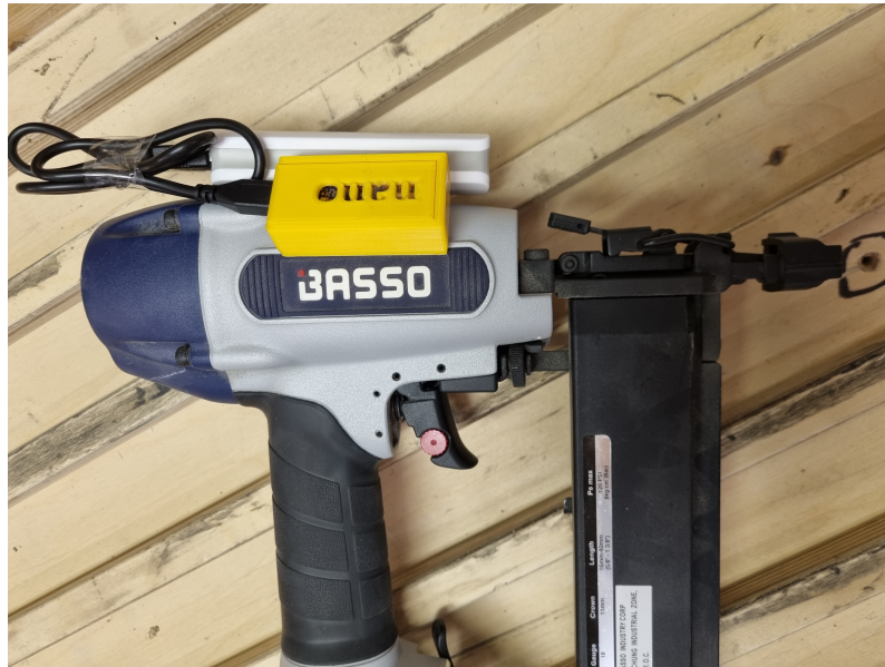
Figure 8: The pneumatic staple gun with the movement measuring Arduino.
