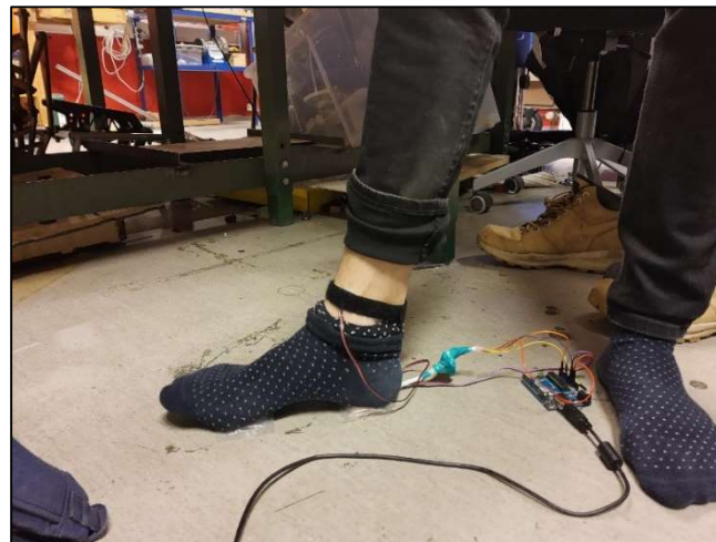
Figure 9 - Setup for testing prototype eight with PPG
