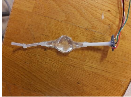
Figure 17 - Updated design of water-filled bladder with BMP388
