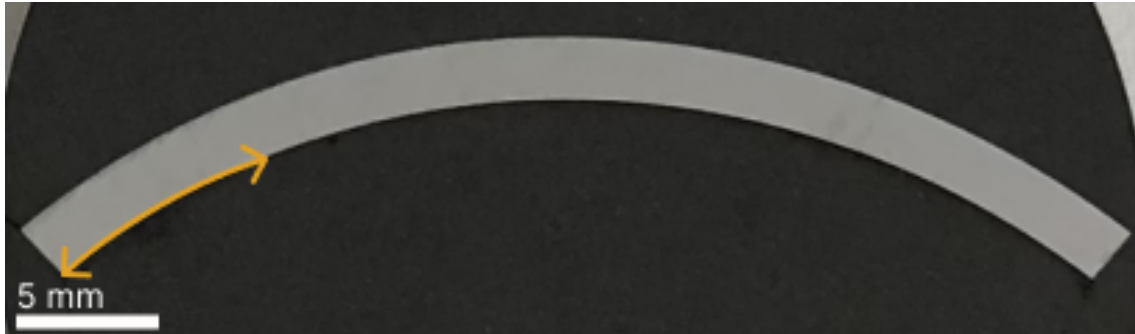
Figure 5.3. Analysed bearing section with orange line showing the area where WECs were observed.
