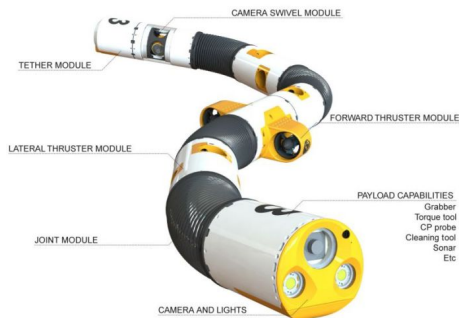
Figure 2.3: A variant of the snake robot Eelume, used as basis for the simulation model.
