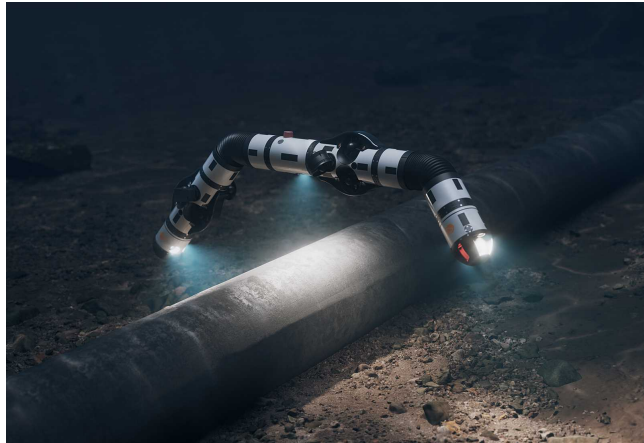
Figure 1.3: An illustration of the Eelume AIAUV investigating a pipe line. Courtesy of Eelume AS
