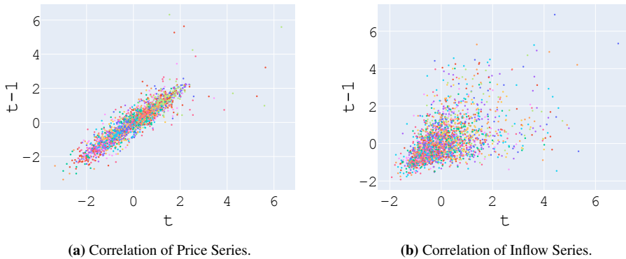
Figure 4.4: Correlation of the Stochastic Data Series, obtained from [7]. The slope of the scattered line is the autocorrelation factor.
