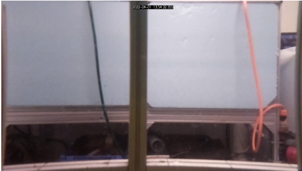
Figure 5.7: Example of pincushion distortion from FISC camera frame.
