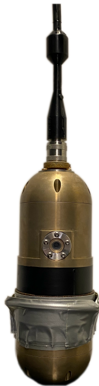
Figure 3.3: Image of FISC capsule with interface cable.
