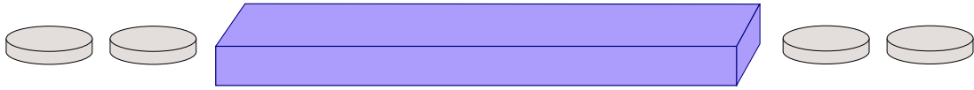
Figure 4.1: Schematic of the ferromagnetically coupled double quantum dot system. The ferromagnet is depicted in blue, with two quantum dots depicted in gray on either end of the magnet, each hosting two spins.
