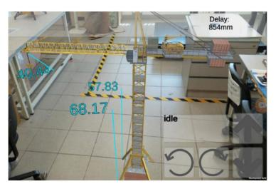
**Figure 4.** The augmented virtual replica that shows the current state of a physical tower crane [35] (licensed under CC BY 4.0). The top-right number indicates the network latency, while the numbers in blue represent the values from a proximity sensor and two force sensors installed on the physical tower crane. The bottom-right buttons can be used to control the physical tower crane.
