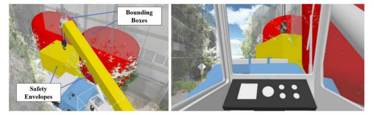
**Figure 8.** The left image shows the view from the observer view, while the right image shows the view from inside the crane cabin [32] (used with permission from American Society of Civil Engineers). The yellow bounding box indicates the minimum safe distance between the lifted load and nearby objects. When a collision is imminent, the red bounding boxes also appear to indicate the area that should not be approached by the operator.
