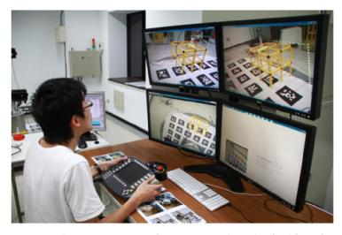
**Figure 5.** The 4-monitor setup for presenting the video feed from four camera views [7] (used with permission from Elsevier). The recommended lifting path (the yellow dotted line) is overlaid into the video feed to help operators avoid collisions.
