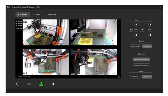
**Figure 3.** The GUI for operating a bridge crane remotely [2] (licensed under CC BY 4.0). The left part shows the video feeds from four different camera views: (**a**) global view; (**b**) cabin view; (**c**) bird view; and (**d**) top view. The right part contains the buttons for controlling the crane remotely. The bottom-left icons could be used to change the input techniques.
