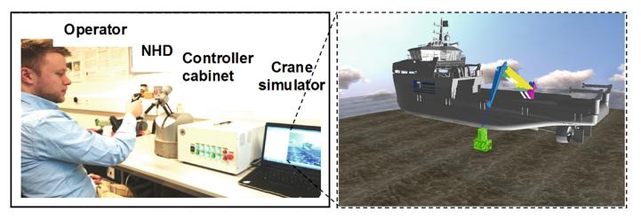
**Figure 7.** The left image shows the haptic device (see "NHD" in the image) that could be used to operate a deck crane remotely and deliver force feedback to the operator. while the right image shows the crane simulator being used in the study [30] (used with permission from Springer Nature).
