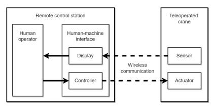
**Figure 1.** Diagram showing a generic interaction between the human operator, the human–machine interface, and the teleoperated crane.
