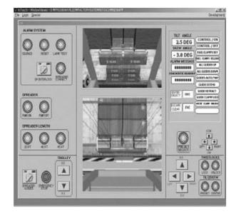
**Figure 2.** The GUI for operating a gantry crane remotely [6] (used with permission from Cambridge University Press). In the middle of the GUI, there are two video feeds, where the upper one shows the cabin view and the lower one shows the spreader view. Both left and right parts of the GUI contain the buttons for controlling the crane.
