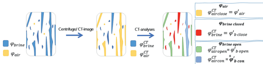
Fig. 3. Classification of pores under in situ conditions after sampling transport centrifuging and CT-imaging and after CT-image analysis.
