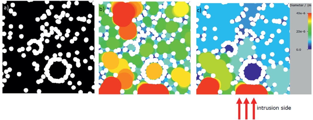
Fig. 3.3 Granulometry and porosimetry used to calculate the pore, and throat size distribution, respectively. a) Shows a structure with the solid material in white and the pore space in black. b) Granulometry: shows the same structure with coloured pore volume. The red volume describes the pore diameters around 40 \mu\text{m} and larger, green areas represent diameters around 20 \mu\text{m} and the blue coloured area below 15 \mu\text{m} . c) Porosimetry: structure shown in a gets penetrated with a non-wetting fluid, indicated by the red arrows. Pores found by porosimetry must be connected to the non-wetting phase. From Linden et al. (2018).
