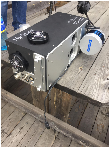
Figure 19: Hyperspectral imaging system Hypsplex Mjolnir VS-620. The same illustration was also used in [1].
