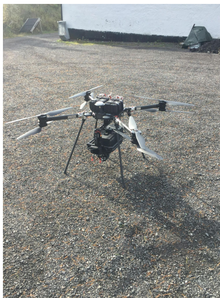
Figure 20: Complete hyperspectral stereoscopic imaging setup, including the octocopter BFD XQ-1400S and the hyperspectral camera rig Hypsplex Mjolnir VS-620. The same illustration was also used in [1].
