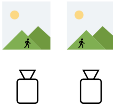
Figure 1: Binocular stereo imaging setup. Two cameras are imaging a common scene from two different points of view, here shifted horizontally wrt each other. By determining the shift, i.e the disparity, of corresponding points in the images, the depth of the scene can be recovered. The same illustration was also used in [1].
