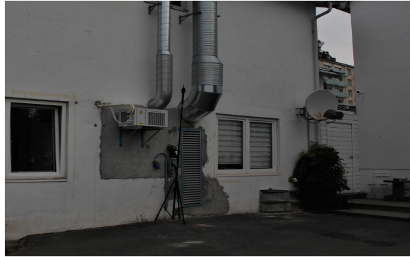
Figure 3.5: Measurement location on the second occasion as the reference receiver point in the noise model.
