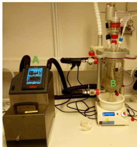
Figure 23: Real-time bioreactor set up showing the temperature controller (A) where deionized water is heated up till 50°C and reactor chamber (B) where the hydrolysis proceeds with monitored temperature and pH.
