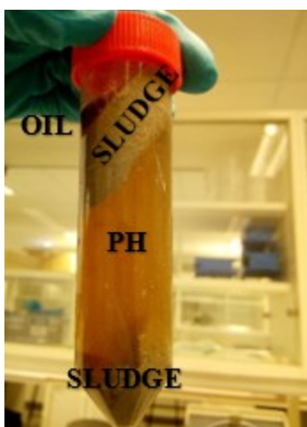
Figure 24: Illustration of the centrifuged protein hydrolysate sample showing the middle clear brownish colored protein hydrolysate (PH), the raw fish meat partly sediment at the top and bottom of the tube, while the lipid was deflected to the upper top left side of the tube.
