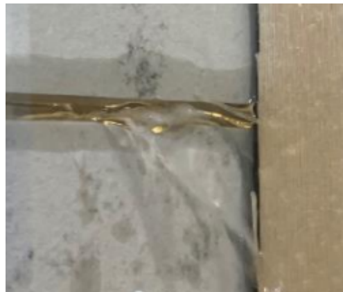
Figure 4.9: Ejection effect from a joint to the wind barrier (Mo & Lid, 2020).
