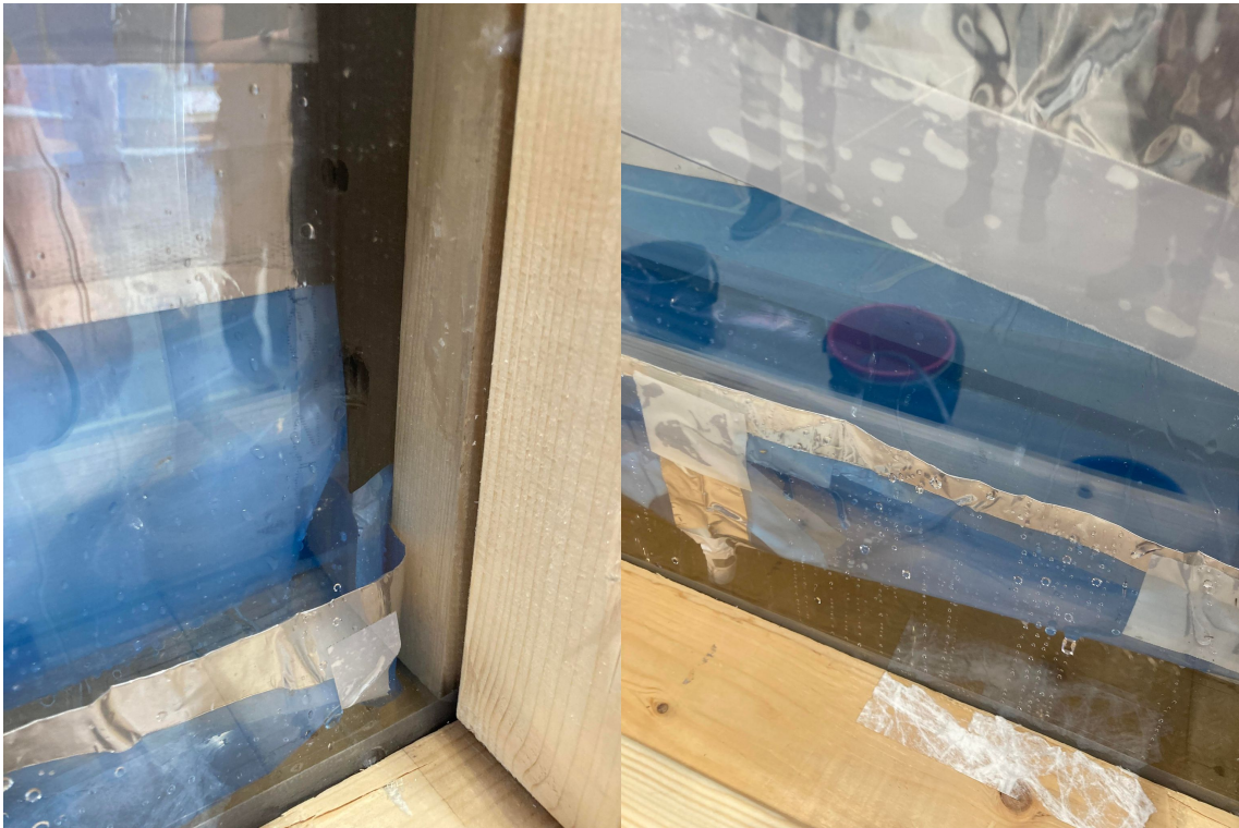
Figure C16: After the test rig is inserted in the driving rain apparatus the double-sided tape is fastened to the Lexan board.
