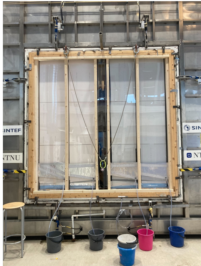
Figure C6: The water in the gutters were led via tubes to buckets, and then measured with measuring cups.
