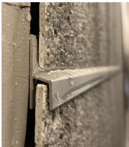
Figure 1.3: A h-profile in a joint. Photo taken during test no. 26 with Glass Fiber Rough and a h-profile.
