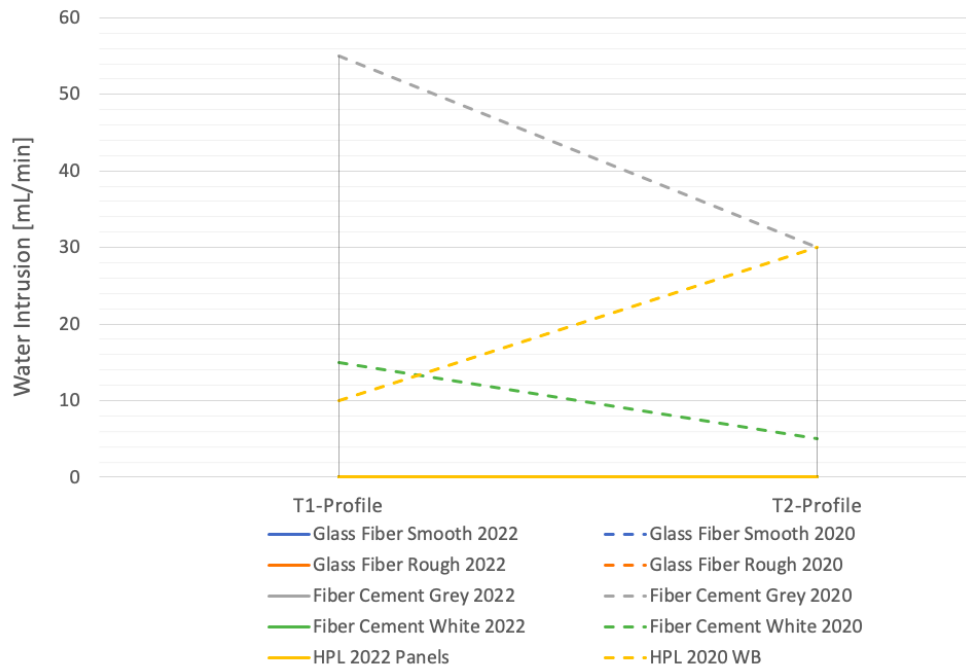
Figure J1: Water intrusion to the wind barrier with the two T-profiles. Comparison between this years laboratory results (2022) and Mo and Lid (2020) results (2020).
