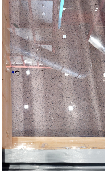
Figure C1: Hole with a diameter of 16 mm drilled through the Lexan board. The hole is drilled 40 mm from the left batten and 220 mm from the bottom horizontal batten. This ensures that the gutter is below the second joint. Four holes in total were drilled.
