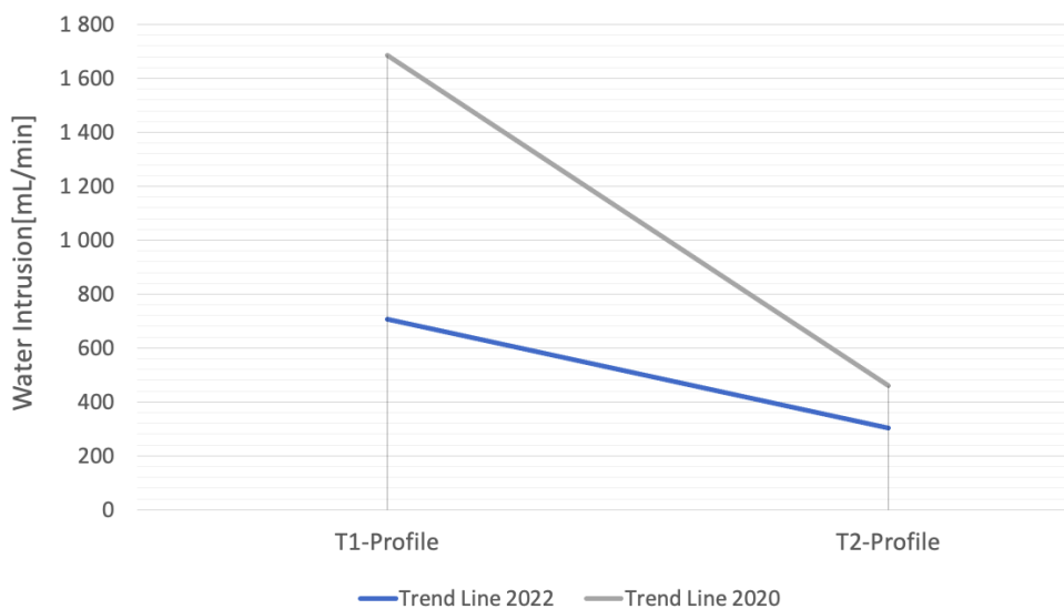
Figure 4.26: Water intrusion to both the wind barrier and interior side of the panels with a T1- and T2-profile. Comparison between the present study’s (2022) results and Mo and Lid (2020) results. The results for the different panels are averaged to give a trend line.
