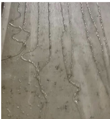
Figure 4.8: Water streams down the interior side of a panel. Photo taken during test no. 97 with Fiber Cement Grey panels and an U-batten.
