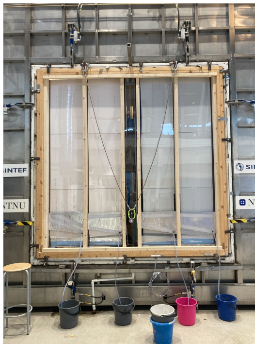
Figure 4. The test rig seen from the interior side. The water collecting system consists of buckets and tubes. Left side of the rig is test section 1, and right side is test section 2.
