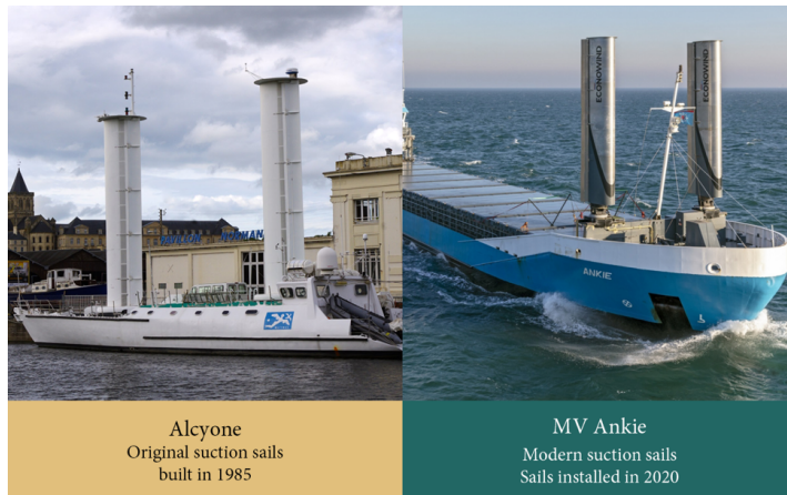
Figure 5: The original turbo sail compared with a modern implementation
