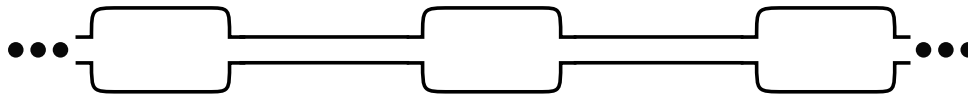
Figure 2.5.1: Chip design with larger chambers connected by narrow channels. The number of chambers vary in the published literature.
