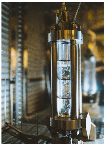
Figure 8: An image of the flotation cell used to conduct the gas flotation experiments
