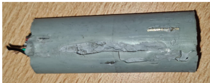
Figure 15.25: Improperly sealed sensor card with Epoxy.
