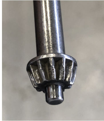
Figure 15.10: Worn drill chuck tool.
