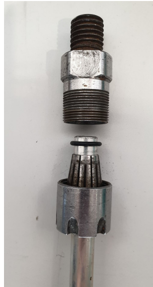
Figure 7.26: Drill pipe arrangement from top: nipple, drill pipe, O-ring, spring collet and collet nut.
