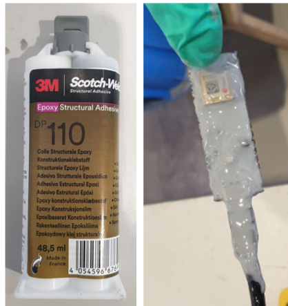
Figure 15.17: Sensor card and cable covered in thin layer of epoxy.
