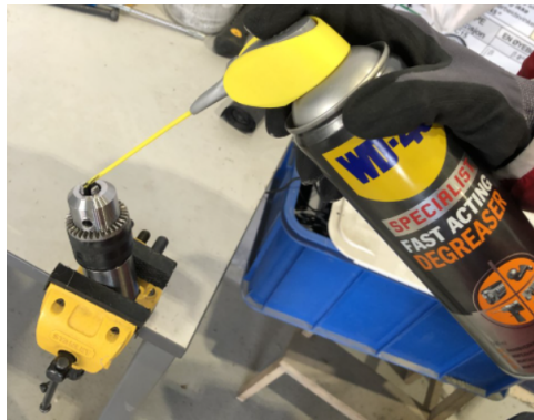
Figure 15.11: Old drill chuck disassembled for cleaning.
