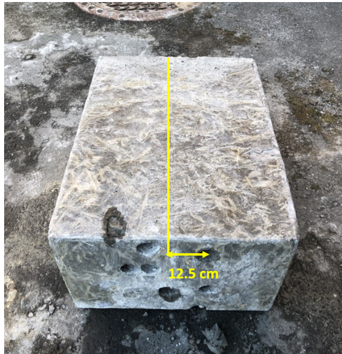
Figure 13.23: Measured horizontal displacement of 12.5 cm when rock sample is tilted on the side.
