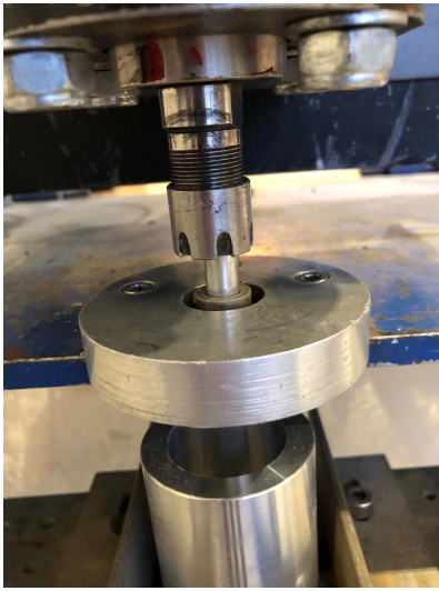
(a) Rig not aligned.
