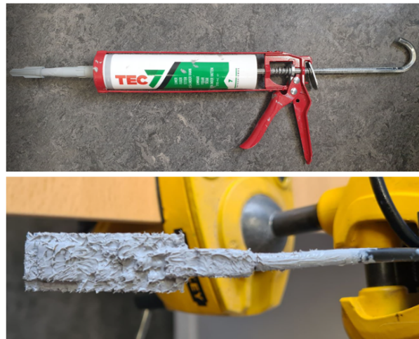
Figure 15.24: Sensor card coated with Tec7 using the dispensing gun.
