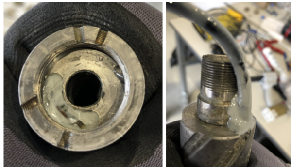
Figure 15.19: Epoxy sealing the sensor card and USB cable.
