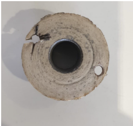
(a) Damaged wear plate after drilling.
