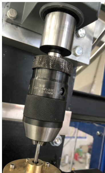
(a) Top drive connection fastening the drill chuck to the top drive motor.
