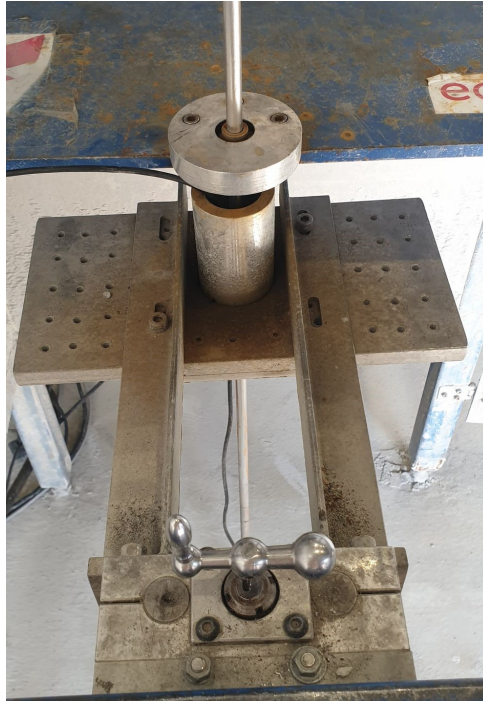
Figure 7.13: Upper and lower stabilizer with manual hoisting mechanism.
