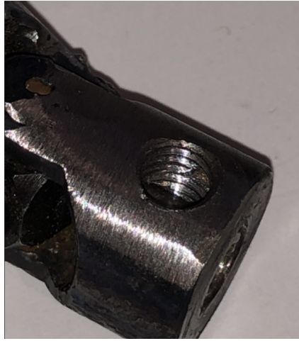
Figure 15.5: New welded threads in the universal joint.
