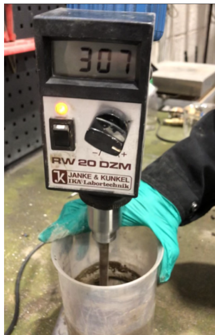
Figure 13.10: Mixing of cement.
