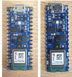
Figure 15.15: Original and guillotine cut sensor card.
