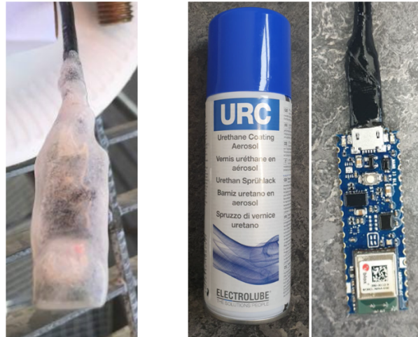
Figure 15.22: Plasti Dip and URC200D coating on sensor card.
