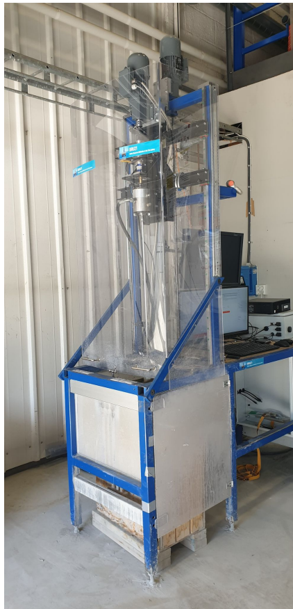
Figure 4.5: Protective cabinet encasing the drilling rig.
