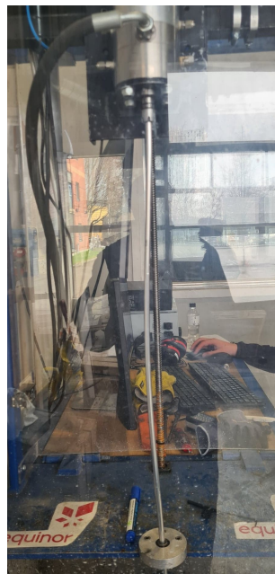
Figure 13.8: Buckled drill pipe.
