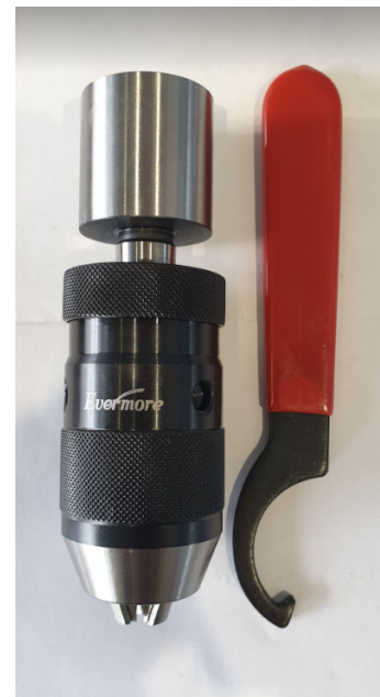
(b) Drill chuck with unique tool.
