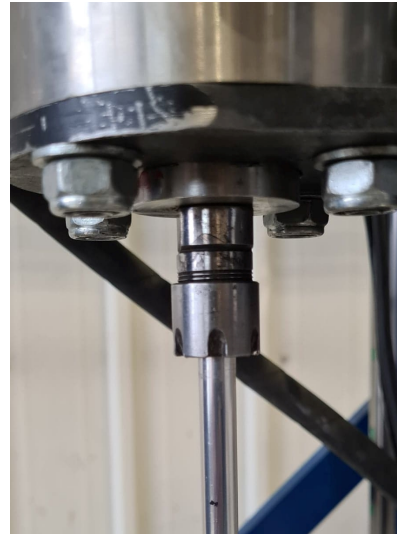
(b) Correct rig alignment
