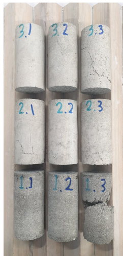
Figure 13.12: Test samples after UCS experiment.
