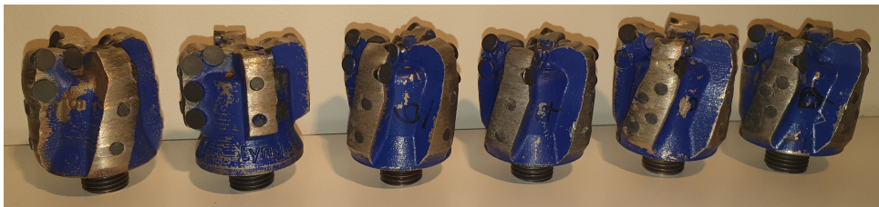
Figure 13.15: State of drill bits after testing.
