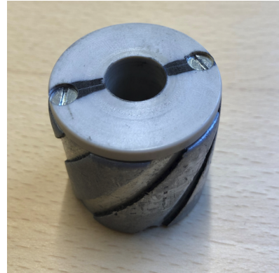
(b) New wear plate installed.
