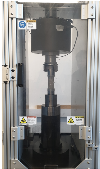
Figure 13.11: RTR-4000 UCS Experimental set up.
