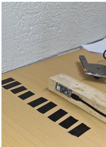
(a) Accelerometer in horizontal position for calibration.
