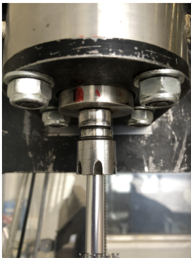
(a) Correct installed drill pipe.
