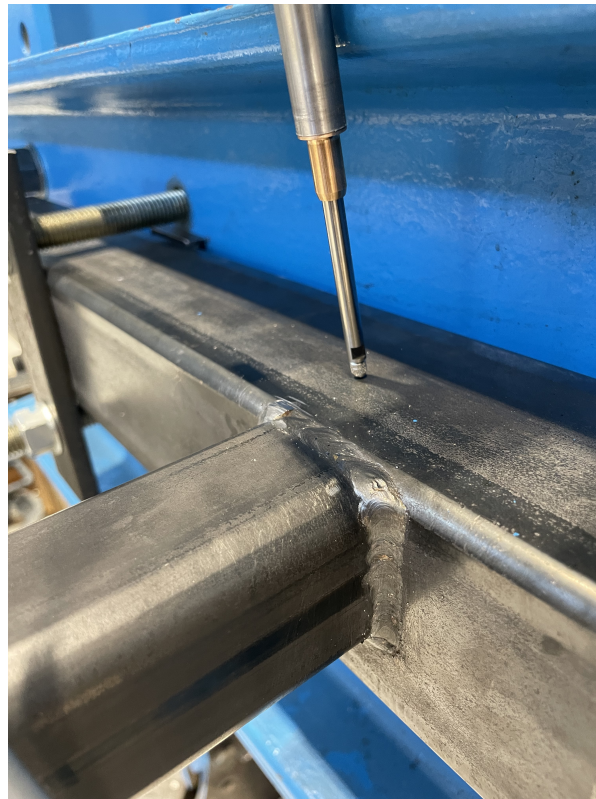
Figure 4.1: Welds between brace and chord, a=3\text{mm}
