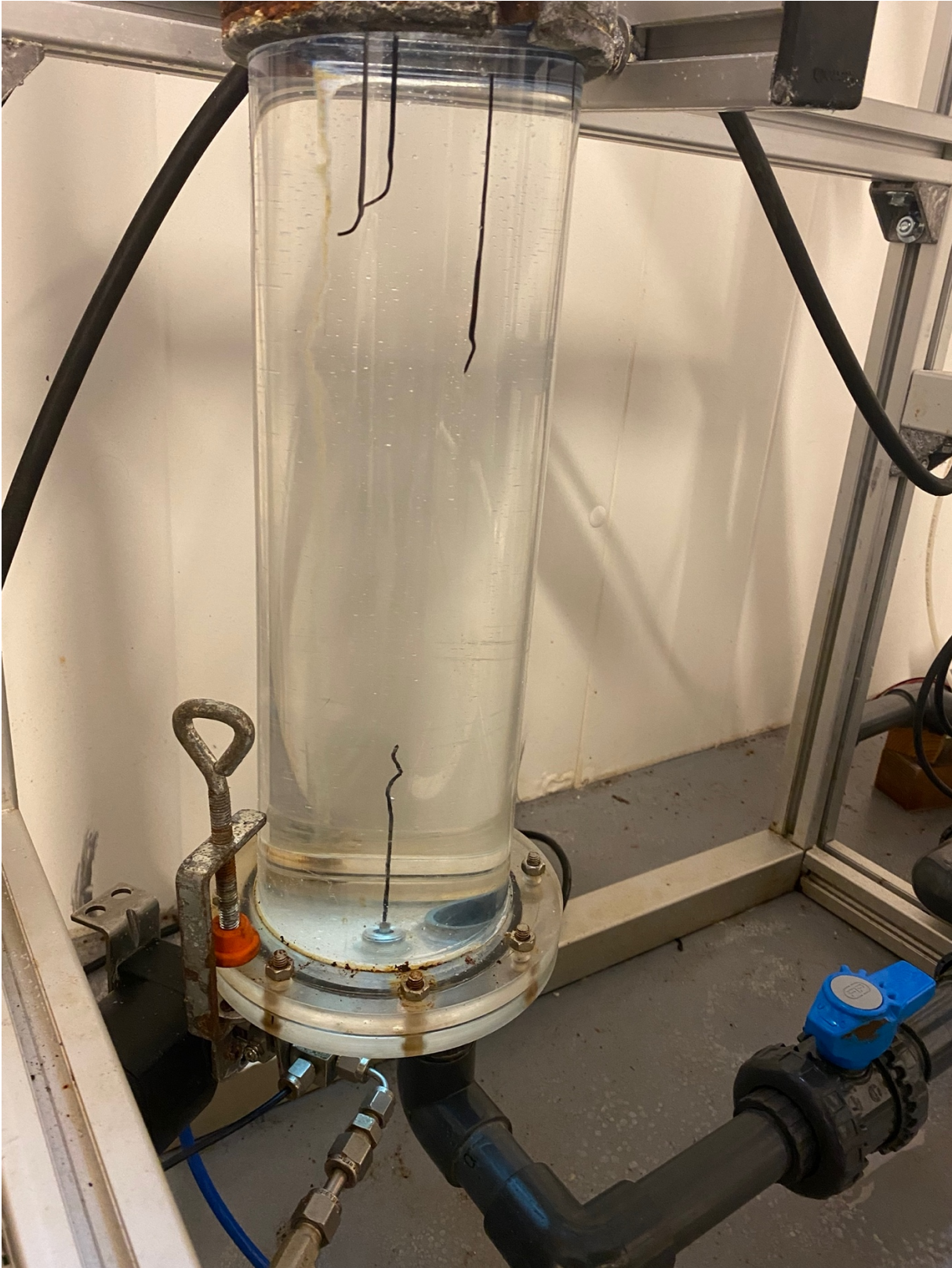
Figure A.1-1: Picture from experiment, where Duva oil was released as a worm, instead of droplets.
