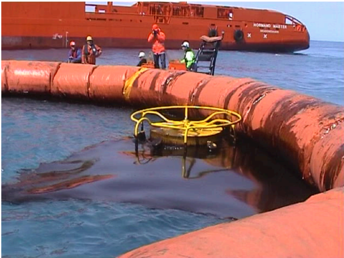
Figure 2-12: Example of a weir skimmer in use. Reposted with permission from Brandvik, P. J. (2020). Oil Spill Contingency methods [Lecture presentation KJ3050]
