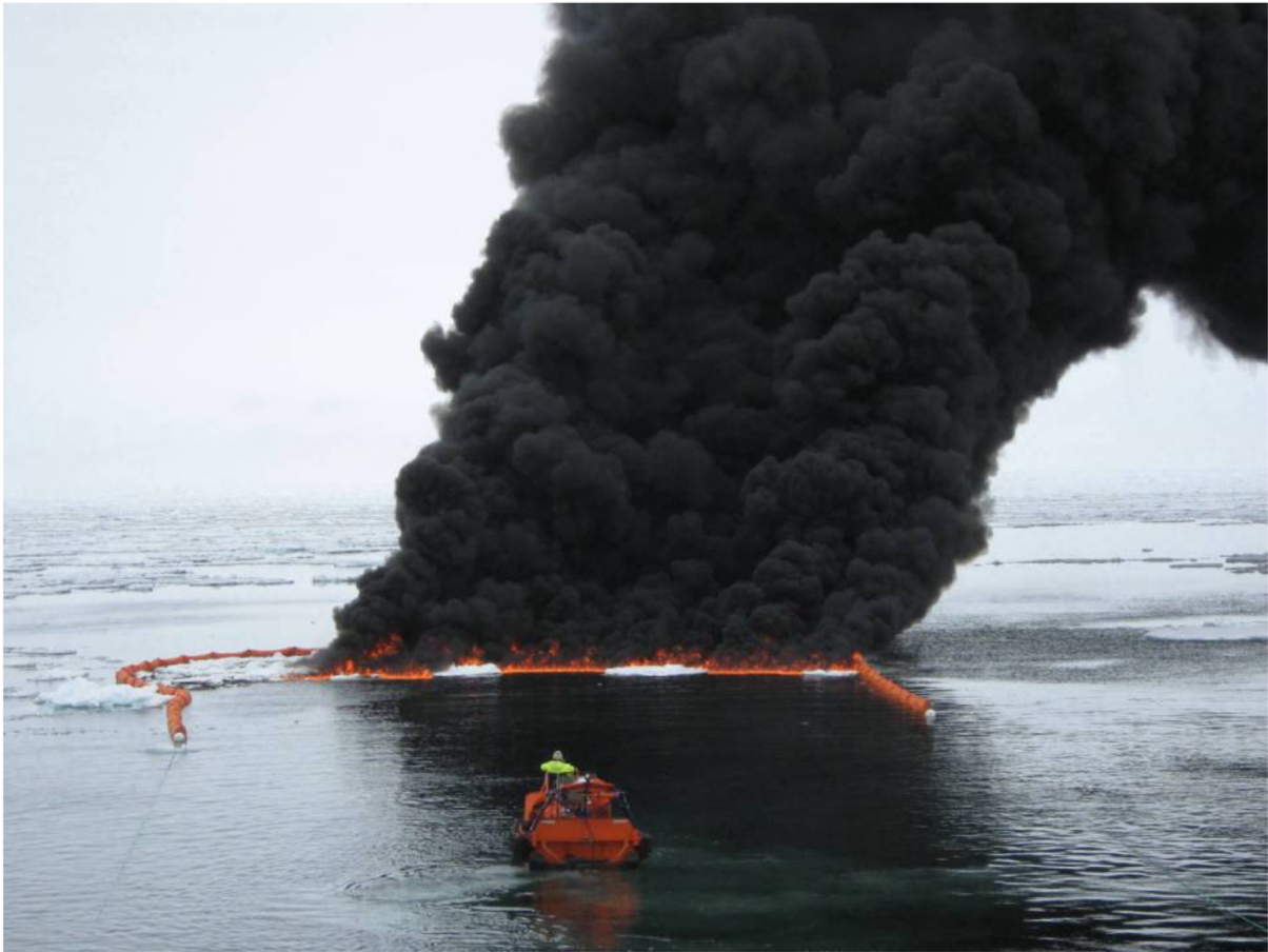
Figure 2-15: Example of in situ burning being tested in the Arctic. Reposted with permission from Brandvik, P. J. (2020). Oil Spill Contingency methods [Lecture presentation KJ3050]
