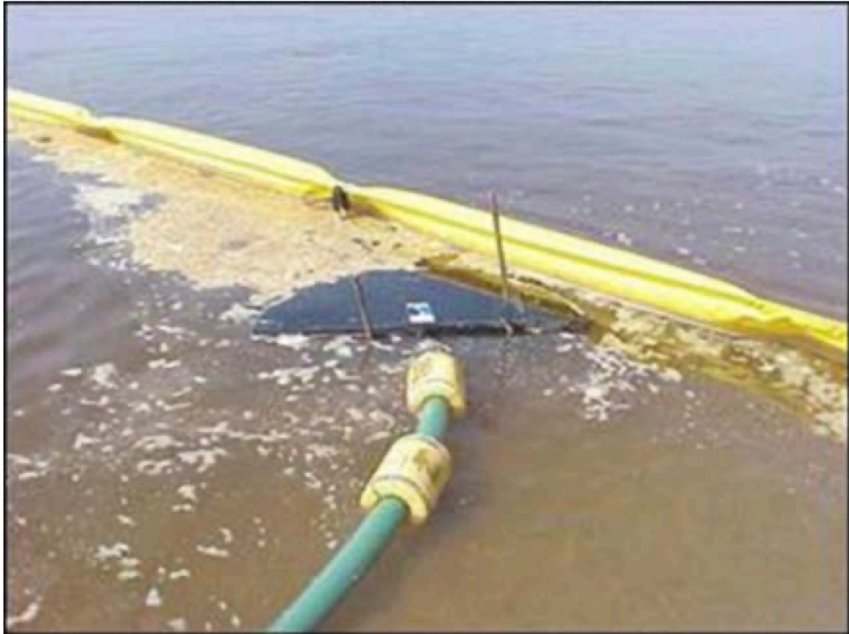
Figure 2-14: An example of a suction skimmer in use. Reposted with permission from Brandvik, P. J. (2020). Oil Spill Contingency methods [Lecture presentation KJ3050] (Brandvik, 2020)
