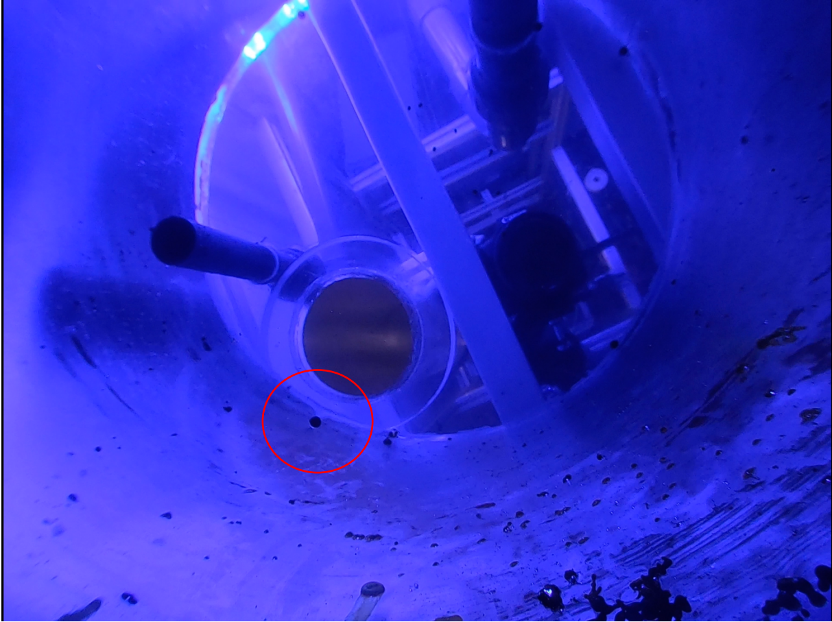
Figure A.4-1: Screenshot from video of solidified droplet taken by GoPro. 1.5mm oil droplet of Duva that have been suspended underwater for 0 min. Droplet is circled in red.
