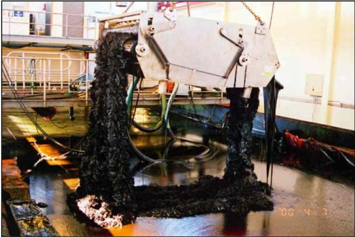
Figure 2-13: Example of an oleophilic skimmer: a Foxtail rope skimmer being tested in a SINTEF laboratory. Reposted with permission from Brandvik, P. J. (2020). Oil Spill Contingency methods [Lecture presentation KJ3050]
