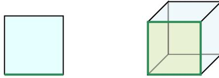
**Figure 2.** Illustration of a face of an element in two and three dimensions.
