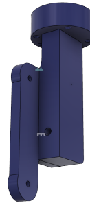
Figure 3.5: Final design end effector with camera mounting.
