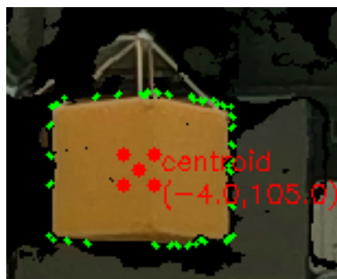
Figure 3.37: Example of five points used to estimate payload position.
