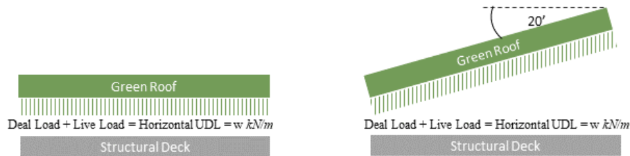
Figure 10: Green Roof Structural Loading
