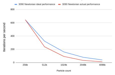
**Figure 6.6:** Ideal performance vs. actual performance in the pool benchmark using Newtonian model with RTX 3090.
