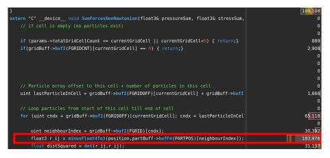
**Figure 5.10:** Output from Nvidia Insight showing source code on the left and number of samples at the right. The samples also records the warp state.
