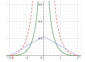
**Figure 3.3:**  $W_{viscosity}$  kernel. The green solid line shows the kernel, the red striped line shows the gradient and the blue dotted line shows the Laplacian. The smoothing radius h is the constant 2.
