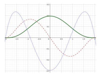
**Figure 3.1:**  $W_{poly6}$  kernel. The green solid line shows the kernel, the red striped line shows the gradient and the blue dotted line shows the Laplacian. The smoothing radius h is the constant 2.
