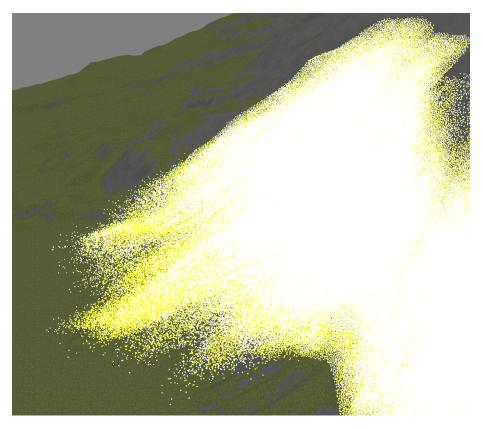
**Figure 6.8:** Color-coded particles that are above the yield stress threshold using the Bingham model. Yellow particles are flowing with reduced viscous stress while the white particles have a high viscosity.
