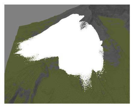
**Figure 6.3:** Avalanche benchmark with 1 million particles after 1000 iterations with the non-Newtonian model using the Bingham model.
