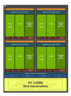
Figure 5.2: Ampere architecture SM design. Used with permission from Nvidia.
