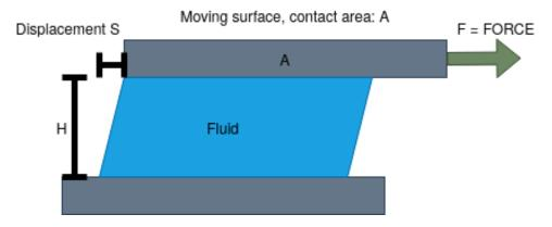
**Figure 2.4:** Illustration of viscous forces on fluid between two plates, inspired by[23].
