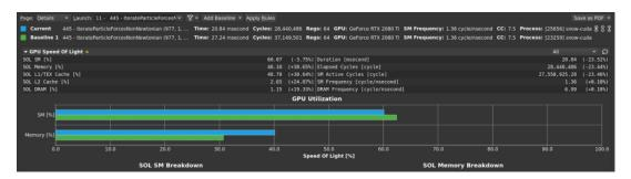
**Figure 5.8:** Speed of light section the IterateParticleForcesNonNewtonian kernel showing GPU utilization. Here one sees one gets a more even memory/compute ultilization ratio, indicating a smaller compute bottleneck.
