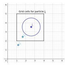
Fig. 3. The grid cell structure illustrated in 2D. The point  $J_i$  represents the current particle. The blue circle represents the smoothing radius.  $J_x$  illustrates other particles in the system.
