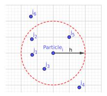
**Figure 3.4:** Mass density approximation for  $particle_i$ . The red striped circle is the smoothing radius. The particles inside the radius will contribute to the mass density of  $particle_i$  based on the distance between them and  $particle_i$ .
