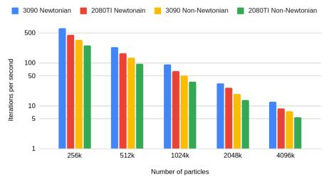
**Figure 6.4:** Pool benchmark results at various particle counts, measured in iterations per second. The same benchmark is run with the Newtonian and Non-Newtonian model on our testing systems.
