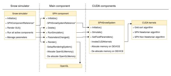
**Figure 4.10:** Diagram that shows how the SPH component is integrated in the HPC-lab snow simulator. Source code is included in the appendices.
