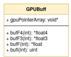
**Figure 4.2:** GPUBuff struct containing GPU memory pointers to particle property buffers.
