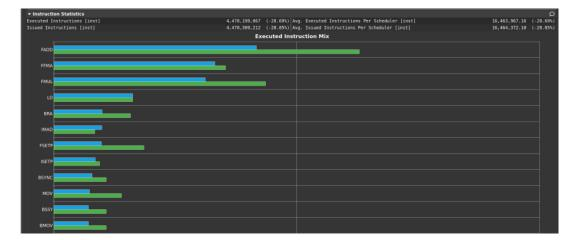
**Figure 5.9:** Instruction statistics for the IterateParticleForcesNonNewtonian kernel. Here one can see that the changes drastically reduced the overall instruction count.
