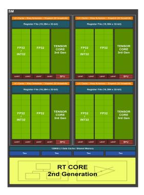
**Figure 2.2:** A image of a single SM unit of the Ampere architecture. With permission from Nvidia.
