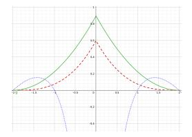
**Figure 3.2:**  $W_{spiky}$  kernel. The red striped line shows the kernel, the green solid line shows the gradient and the blue dotted line shows the Laplacian. The smoothing radius h is the constant 2.
