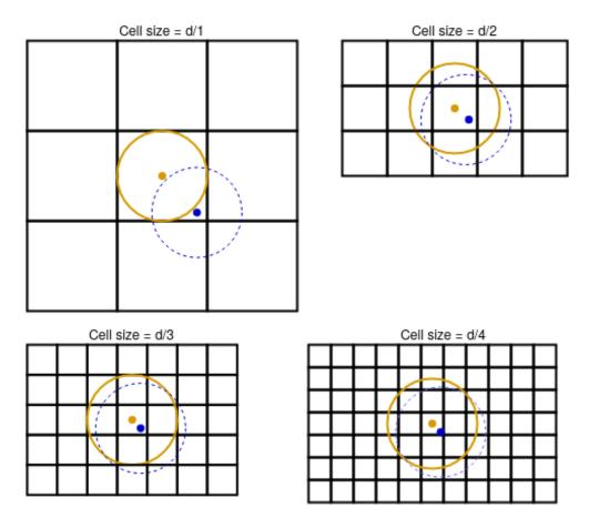
**Figure 4.3:** Figure of several 2D grid cell sizes with a constant particle influence *diameter*.
