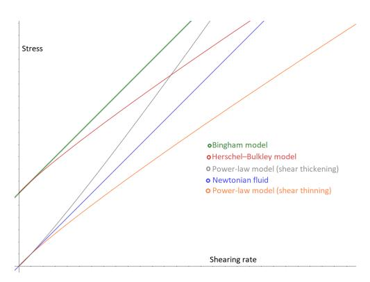
**Figure 2.5:** Rheological models viscosity illustrated at different stress and shearing rates. Inspired by[23].
