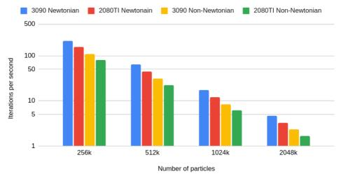
**Figure 6.5:** Avalanche benchmark results at various particle counts, measured in iterations per second. The same benchmark is run with the Newtonian and Non-Newtonian model on our testing systems.
