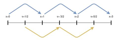
**Figure 4.4:** Leapfrog time integration. Velocity calculated at every half step and position is updated at every full step
