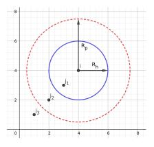
Fig. 2. Verlet list search radiuses illustrated. The red dotted circle represents the buffer radius  $R_p$  and the solid blue circle  $R_h$  represent the smoothing radius. The center of the circles is the particle *i*. There are also some surrounding particles  $j_x$  in different areas.
