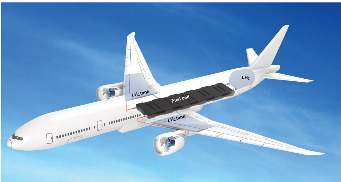
Figure 1: Conceptual airplane with fuselage-integrated fuel cells and LH 2 tanks and additional wing-embedded LH 2 tanks.
