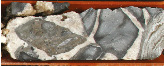
Figure 2.3: Core plug sample photo of angular breccia. Interval of cave roof collapse. Loppa High region.
