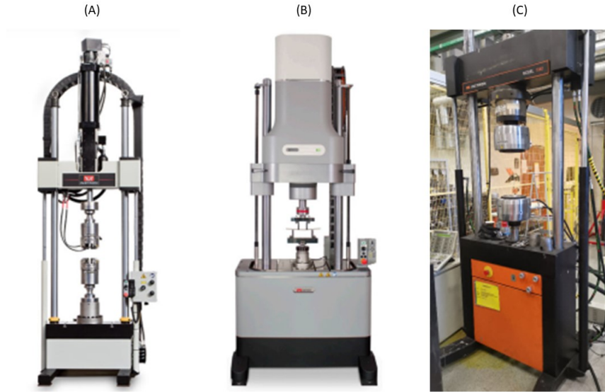
Figure 11: (A) Instron 8854 - 250KN, (B) Instron Electropuls - 10KN and (C) Instron 1342 - 100KN
