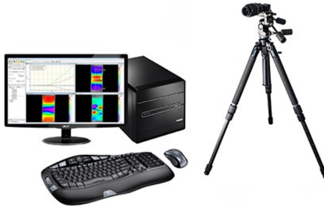
Figure 10: DIC VIC-2D measurement system [4]
