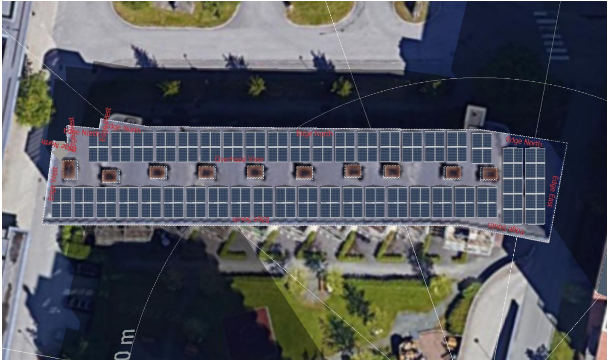
Figure 4.2: The EW PV system as seen from above. Image created in PV*SOL.
