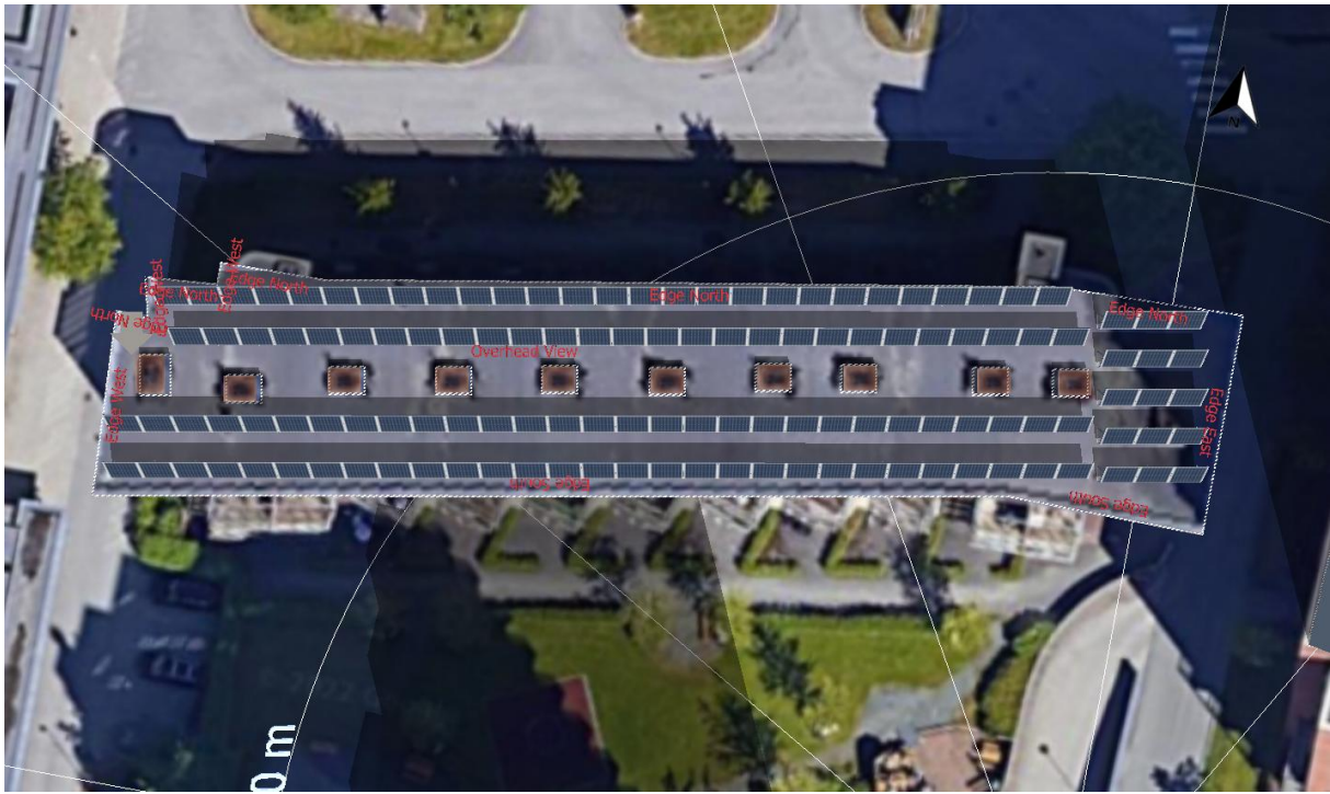
Figure 4.1: The south-oriented PV system as seen from above. Image created in PV*SOL.
