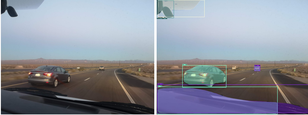
Figure 5.6: Image Segmentation by the Tensorflow's implementation of Mask R-CNN (He et al., 2017). Photo taken by the author.
