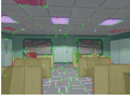
Figure 5.2: RViz visualization of Semantic-Kimera-VIO run on the uHumans2 office 0h dataset. The visualization shows the semantic segmentation image overlaid with the debug feature tracking image using the jsk_rviz_plugins
