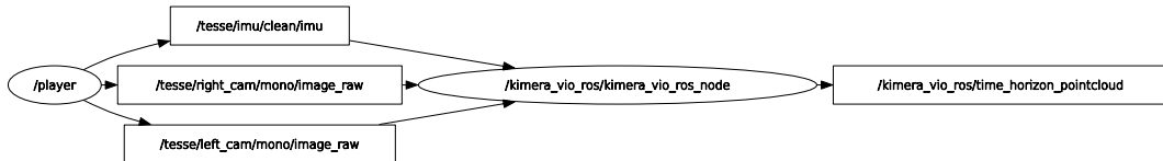
Figure 5.9: The ROS architecture of the original Kimera-VIO with all relevant ROS nodes (circles) and topics (rectangles). The figure was created using ROS rqt_graph .
