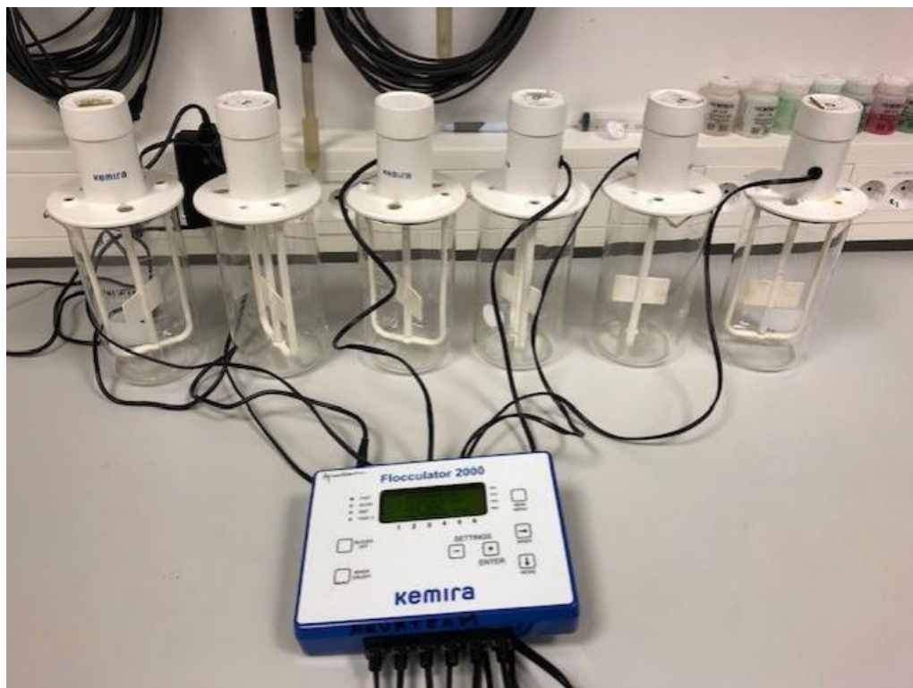
Figure 15: The figure shows the setup of the jar apparatus Kemira Flocculator 2000. [6]
