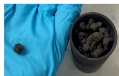
Figure 14. Molybdenum crucible filled with a sintered sample.
