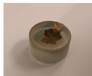
Figure 15. A gold-coated sample of reduced pellets.
