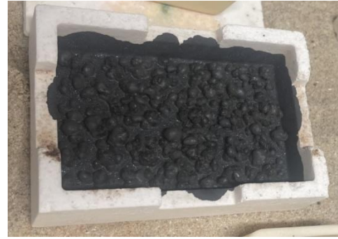
Figure 19. The smelted sintered pellets.
