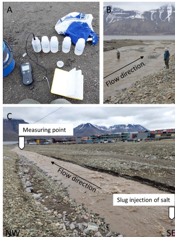
Figure 19 The salt dilution method in Longyearelva for discharge calculations. A) Calibration of electronic conductivity (EC) meter. B) Measuring the EC in the river. Photo by Aga Nowak. C) The long, unbraided stretch of Longyearelva by Polarriggen, where slug injections of salt and the measuring EC were made.
