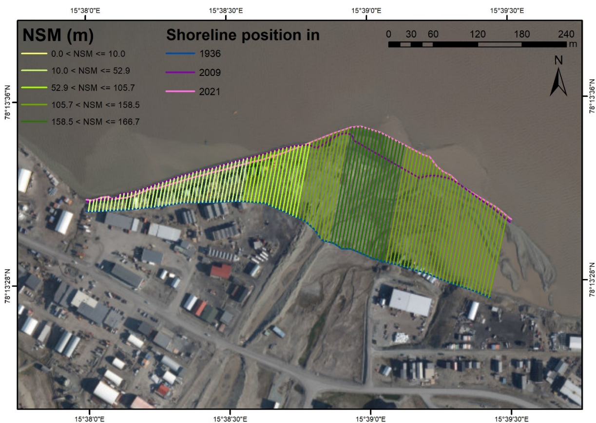
Figure 51 Net Shoreline Movement (NSM) of the Longyear delta from 1936 to 2021. Generated using Digital Shoreline Analysis System (DSAS) with shorelines drawn from orthophotos and aerial imagery. The shorelines from the years 1936, 2009, and 2021 are included. The background is the 2009 orthophoto3.
