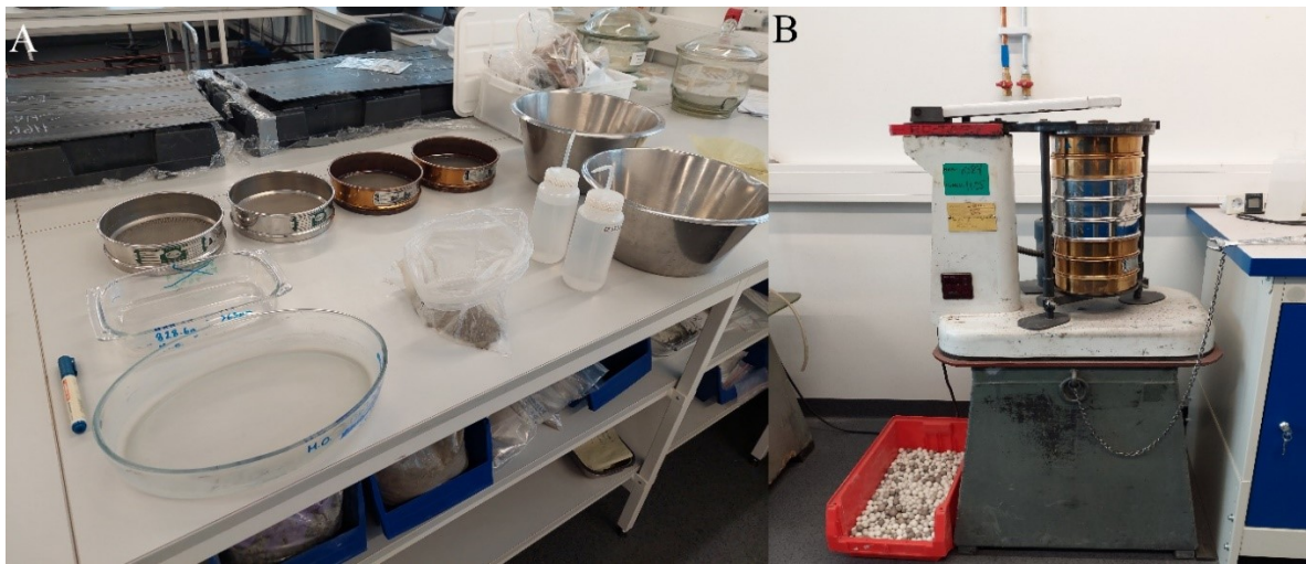
Figure 24 Sediment samples collected from the Longyear delta were first (A) wet sieved and dried, and then (B) dry sieved.
