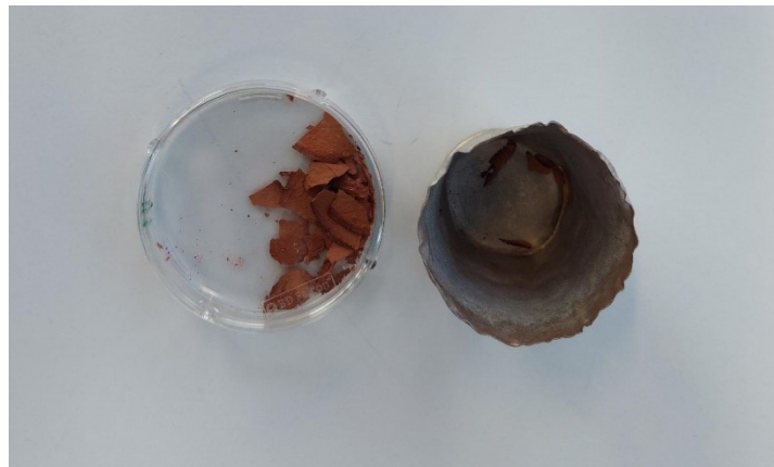
Figure 22 From the failed attempt to incinerate the filter paper to access sediments for further analysis.
