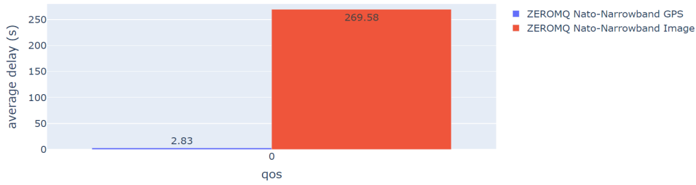
Figure 52: Average delay using the NATO Narrowband network model
