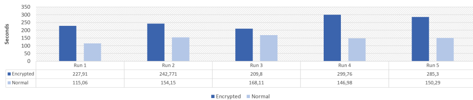
Figure 8.17: Comparison of performance with and without server-side encryption enabled with Azure cloud storage. The values in the table right beneath the bars show the actual value in seconds it took to finish the execution of the said operations.
