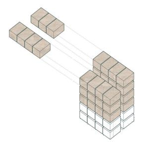
lining on one side and Modules fully finished on all sides with integrated services (Built Offsite, 2016). Generally, prefabricated prefinished modules are able to support their own weight without an additional load bearing structure, but in other cases, modules are designed to support 4 levels of modules stacked on top of each other without the need for a Structure such as Treet example.
