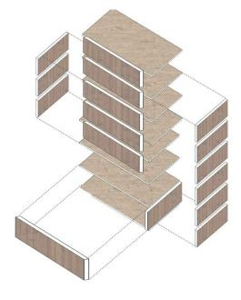
them in the manufacture. The Australian residential building Forte (2012) has a structure that rely completely on the CLT panels that can support their own weight.
