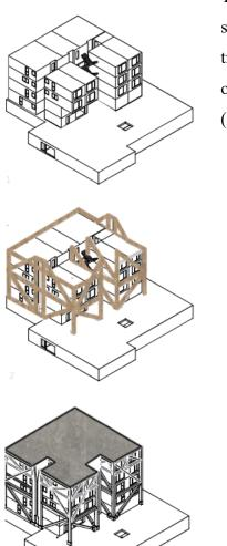
The roof is also a prefabricated and element-based concrete slab. The concrete slabs are incorporated to connect the trusses, but an additional main function is to increase the mass of the building and hence to improve the dynamic behavior (Bjertnæs and Malo (2014).
