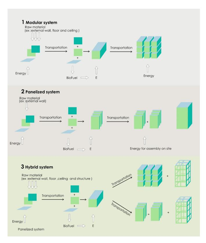
Figure 10 :prefabrication application different production and installation process
