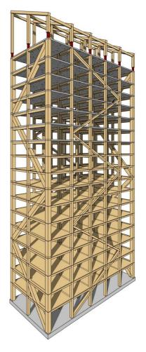
Figure 23 Structural system of Mjøstårnet
