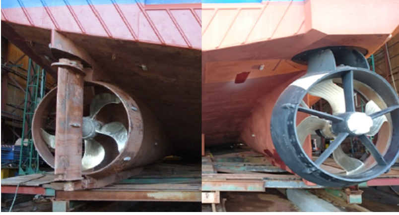
Fig. 2. The propulsion arrangement before and after retrofit.
