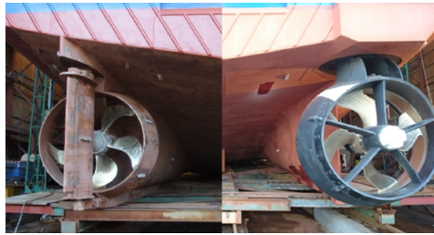
Figure 2.11: The propulsion arrangement of the R/V Gunnerus before and after retrofit.
