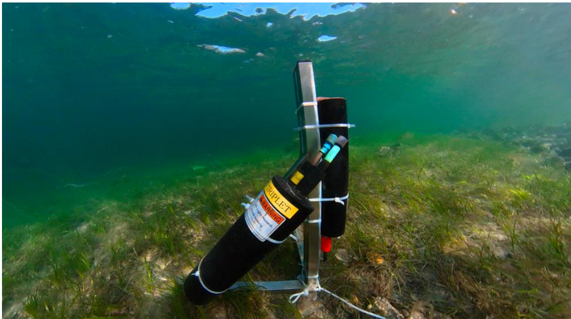
Figure 2.4: The set-up of ECO Triplet sensor and the spectroradiometer at the examined seagrass meadow in Hopavågen. With the first sensor measuring the concentration of phytoplankton (Chl a ), colored dissolved organic matter (cDOM), total suspended matter (TSM), and the latter measured depth and downwelling spectral irradiance ( E_d(\lambda) ). The sensors ran for 24 hours. Photo: G. Johnsen.
