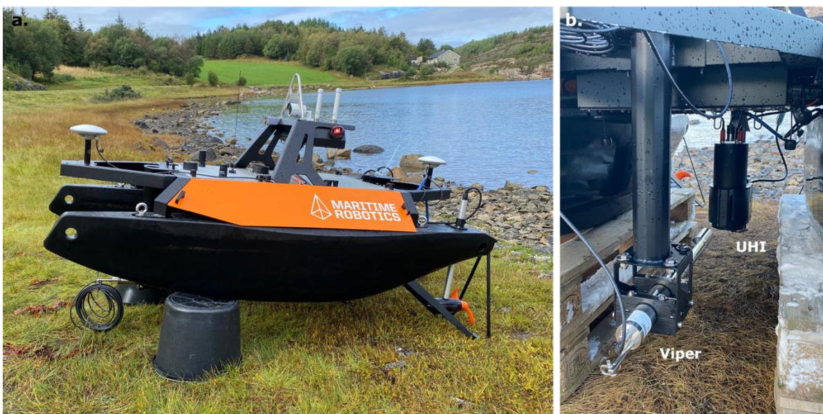
Figure 2.2: The Otter Pro prior to deployment at the study area in Hopavågen (a). Close up and positioning of the USV payload; Viper and UHI-4, attached by custom made metal brackets. Photo: M. Søreng.
