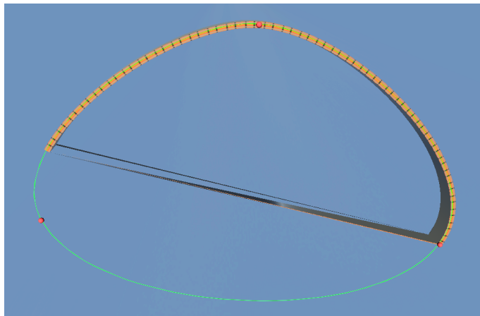
Figure 33: Rail mesh breaking after exceeding a certain distance
