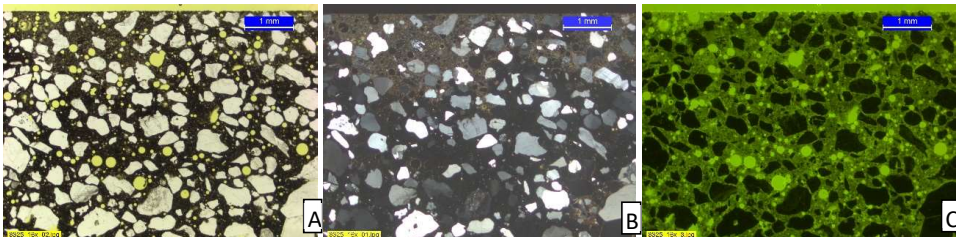
Figure 6: Picture of area in concrete 25FA with representative carbonation in the three modes polarized light (A), X-polarized light (B) and Fluorescence (C). Concrete exposed for 8 years in urban environment. Exposed surface pointing upwards.
