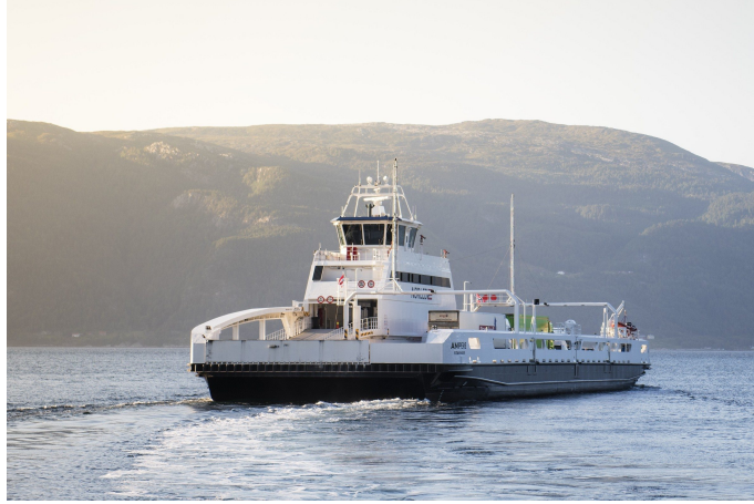
Figure 2.2: The worlds first electric passenger ferry, Ampere . [13]
