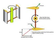
Figure 29: How the Darrieus turbine work [22]
