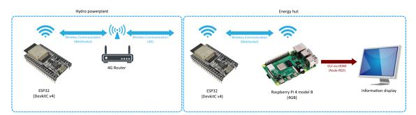
Figure 49: General overview of the electronic setup
