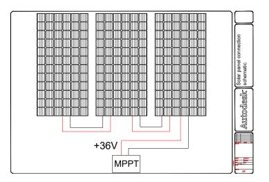
Figure 14: Solar panel schematic connections
