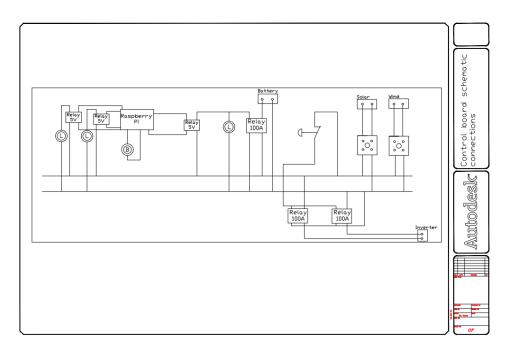
Fig 2: The Energy Hut's control board schematic.
