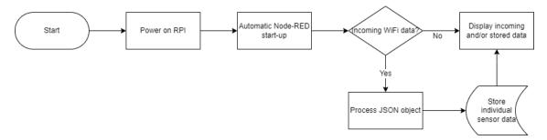
Figure 53: Flowchart for the RPI with Node-RED
