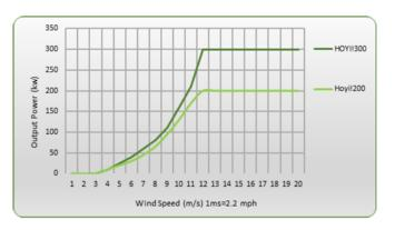
Figure 37: Power to wind curve of Hoyi wind generators [25]
