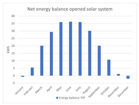
Figure 12: Energy balance forecast in the opened position
