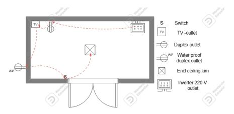
Figure 7: AC 2D-wiring diagram for Energy Hut
