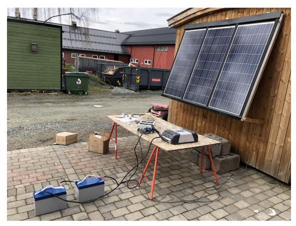
Figure 23: Testing of the MPPT and inverter
