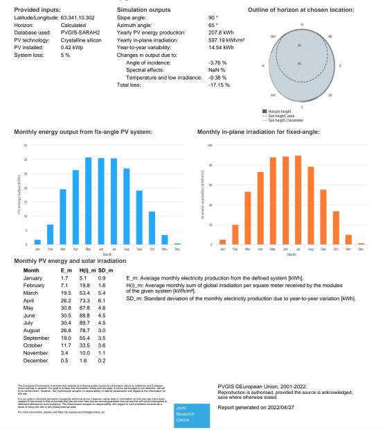
Figure 70: Program result for the solar energy forecast in the "closed position"
