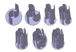
Figure 28: Examples of Savonius turbine designs [20]
