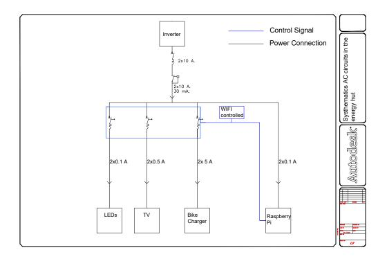
Figure 8: AC diagram for Energy Hut
