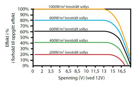
Figure 15: Voltage-power curve for the solar panels [9]
