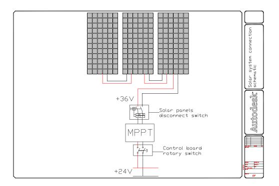
Figure 21: Solar system schematic connections
