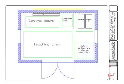
Figure 4: Energy Hut Layout top view
