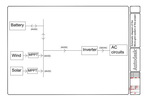
Figure 2: Schematic design of our micro-grid system
