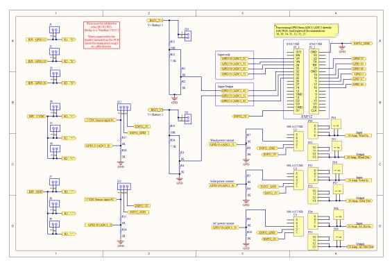
Figure 50: The groups design of the wiring schematic for the PCB  $\,$
