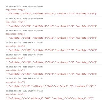
Figure 67: Data transmission test with potentiometer, from full actuation down to no actuation. Change can be seen in "voltData\_1" going from full 12 bits down to 0.
