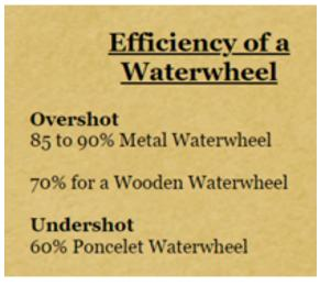
Figure 72: Efficiency of waterwheels [34]
