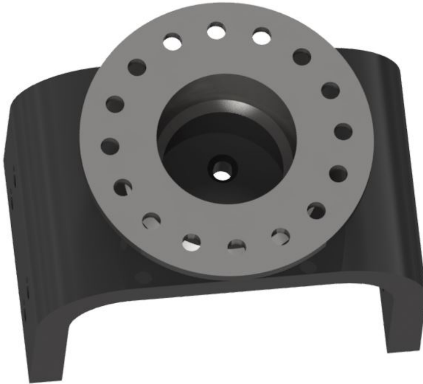
Figur 40: Dreneringshull i opplagring.
