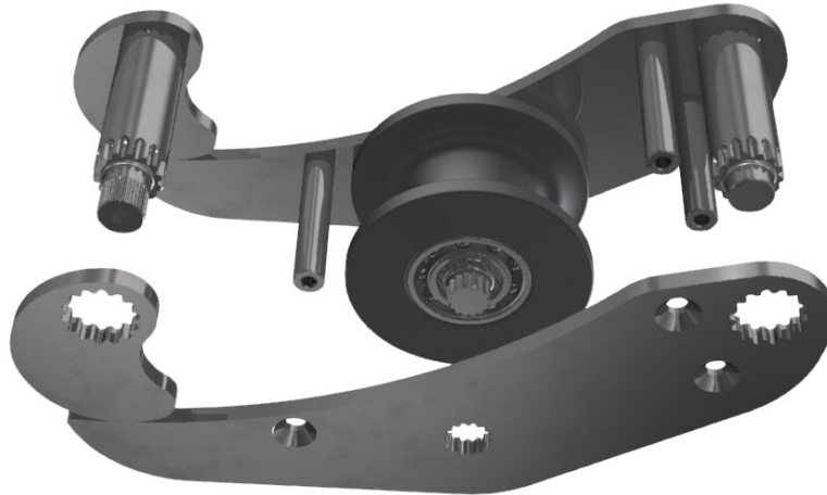
Figur 26: Mekanisme for beltestramming.
