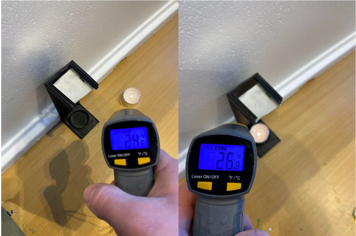
Figur 28 Materialet papp testes (foto: Fliflet-Jacobsen, 2022)
