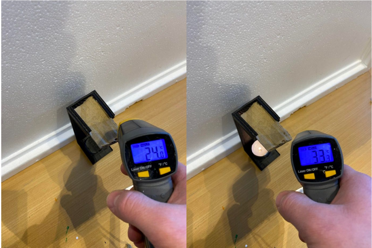
Figur 28 Materialet papp testes (foto: Fliflet-Jacobsen, 2022)
