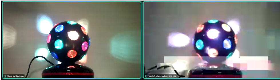
Figure 6.5: A screenshot of a video feed with block artifacts on the right, taken during latency testing scenarios.
