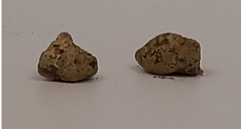
Figure 11: White inclusions found in the polymetallic manganese nodules.
