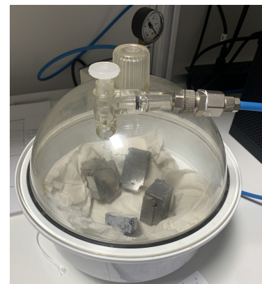
Figure 3.13: Vacuum drying of samples after being submerged in ethanol for at least 24 hours.
