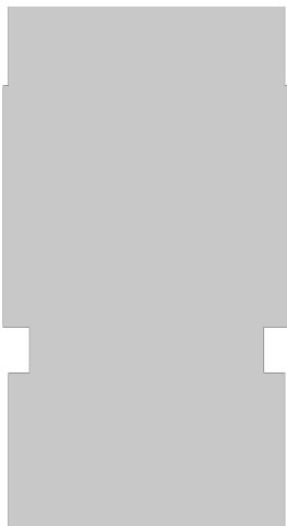
Figure 3.16: The outline of the 2D-COMSOL Multiphysics® model. In this figure a subsection of the whole system is shown, where the filter house is shown with the inlet and outlet tube on both sides. The flow goes from top to bottom, and the voids in the filter house next to the outlet tube represent the protrusions in the filter house.
