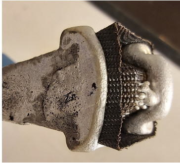
Figure 4.31: An unsuccessful casting of metal. The molten metal was able to penetrate the weaves but solidified before fully submerging the filter.
