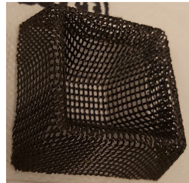
Figure 1.1: A geometrical shaped filter (20x43L) of the type Rigid Glass Weave. This type of filter is a sheet-like filter, its structure does not have an impact on tortuosity.
