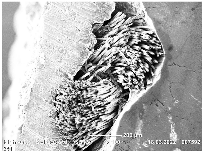
Figure C.22: Close-up of a weave, cavities caused by casting shrinkage and possible permeation of ethanol in the sample of geometrical shaped filter PO48 - 25054 (20x43L). Zoom = x100. SEI. High-Vacuum.
