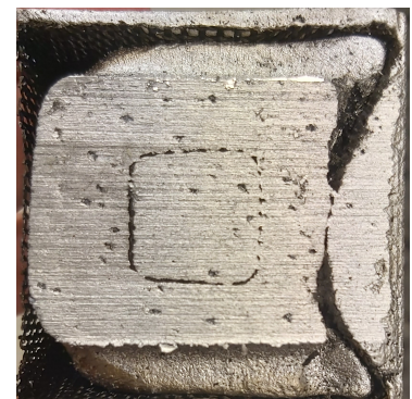
Figure 4.30: Successful casting of metal. The molten metal was able to penetrate the weaves and fully submerge the filter before solidification.
