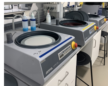
Figure 3.12: The polishing machines used for diamond polishing of the samples, ATM Saphir 350.
