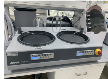
Figure 3.11: The polishing machines used for grinding and polishing of the samples, ATM Saphir 360.
