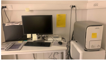
Figure 3.15: Setup consisting of the JEOL JCM-6000 scanning electron microscope, computer and display monitor.
