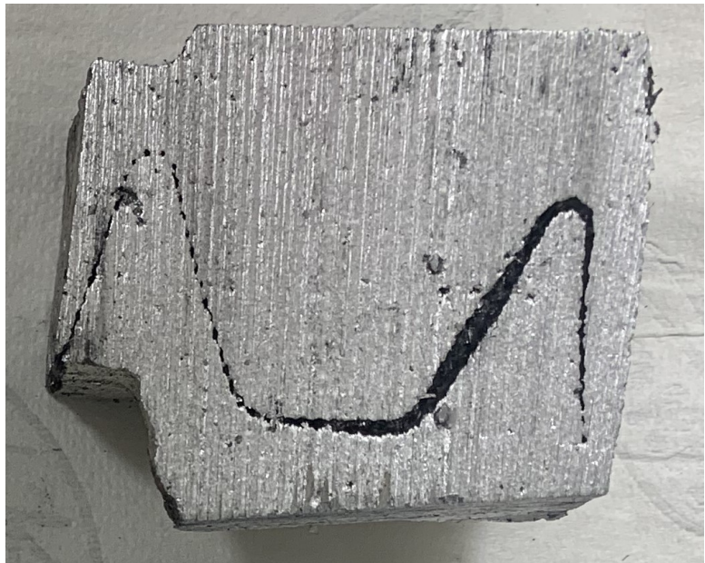
Figure B.4: Cut casting sample of PO48 - 2505X (20xXW2) before metallographic preparation for SEM
