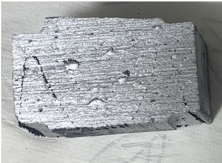
Figure B.2: Cut casting sample of PO48 - 25653 (20x40L) before metallographic preparation for SEM
