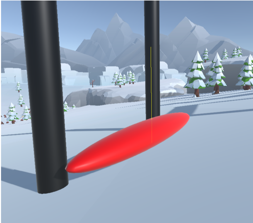
Figure 3.2: An image of a movement node. The yellow line here represents how the nodes has adjusted itself based on the current terrain.
