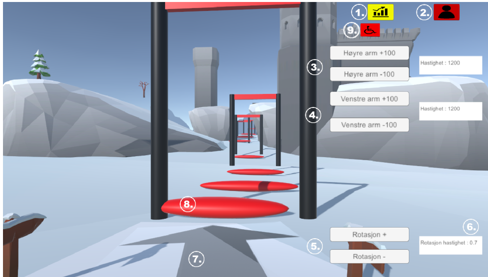
Figure 3.7: Image of the UI with displayed while a player plays in the background. 1: Statistic panel, 2: Enable/disable UI, 3: buttons to increase/decrease right arm assistance, 4: buttons to increase/decrease left arm strength, 5. buttons to increase/decrease rotation speed of wheelchair, 6: panel to show current speed of variables, 7:arrow decal as discussed earlier in chapter 3 , 8: The red cylinders here represent the movement nodes, 9: button to toggle wheelchair mode
