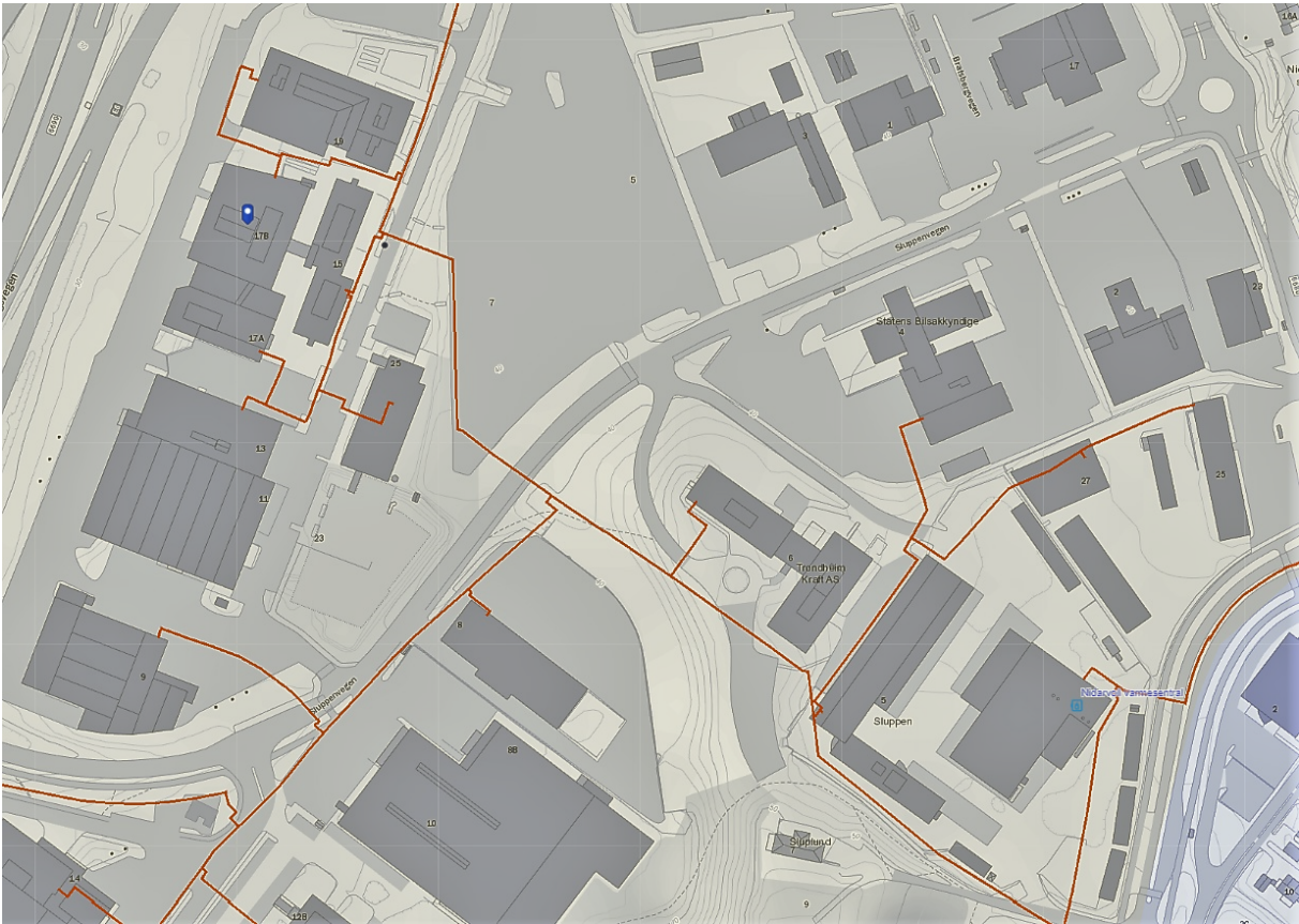
Figure C.1: Map of the district heating distribution at Sluppen, and the nearby heating plant at Nidardvoll [111].
