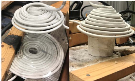
Figure 13: Pancake coil and an insulated graphite mould at 750°C placed in the coil.
