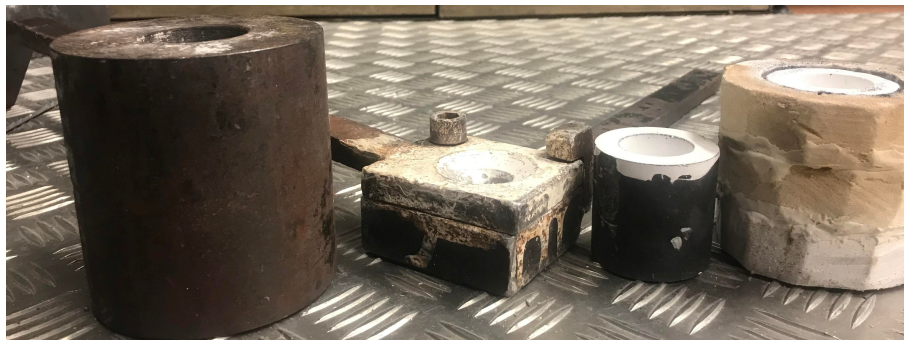
Figure 12: Left to right: cylindrical iron mould, RSD iron mould, heated graphite mould at 250\text{ }^\circ\text{C} and insulated heated graphite mould at 650\text{ }^\circ\text{C} .
