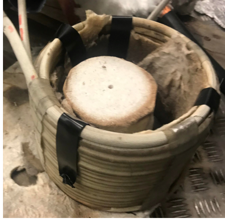
Figure 14: Insulated graphite mould heated to 750°C placed in the round coil.
