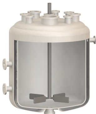
Figure 7: Industrial stirred tank cross-section[11]
