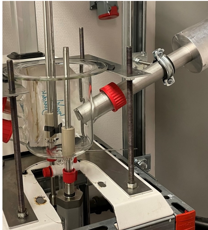
Figure 18: Stirred Tank Cell system close-up
