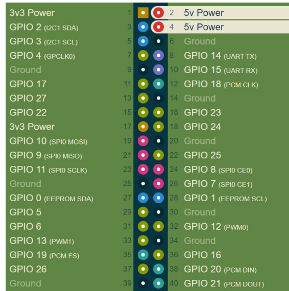
Figure 50: Overview of the Raspberry Pi's GPIO-pins.
