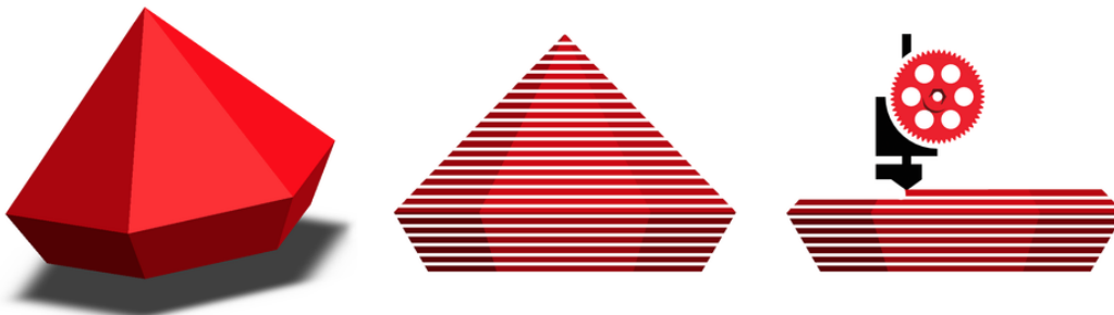
Figure 3: Slicing process [10]. From 3D model to sliced 3D model to 3D model being printed one slice at a time.
